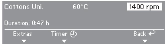
Turn the multi-function selector to highlight programme, temperature or spin speed. Pressing the multi-function selector selects the highlighted option and opens the relevant sub-menu.
