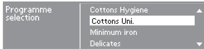
You can use the multi-function selector to select any programme. The highlighting will move up or down depending on the direction the multi-function selector is turned in.
