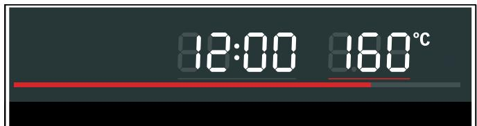
**Note:** Due to thermal inertia, the actual temperature inside the cooking compartment may be slightly different to the temperature that you set.
